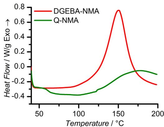
**Figure 2.** Assessment of the conditions used to cure **2** and NMA to produce Q-NMA, with evaluation of heat flow versus temperature by DSC.
