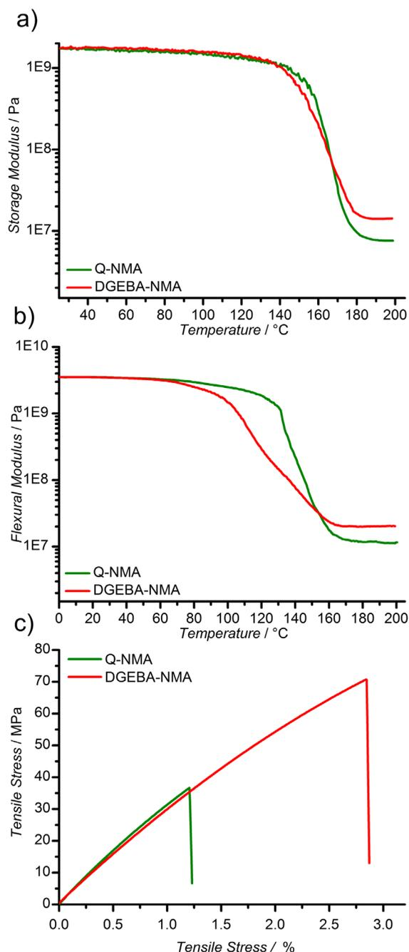
**Figure 4.** (a) Tensile storage modulus as a function of temperature. (b) Flexural modulus as a function of temperature. (c) Representative stress–strain behavior ( $n = 5-6$ ).
